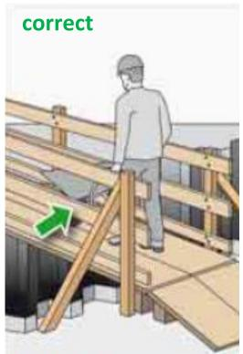
In case of open excavations create safe passages between excavation trenches!
