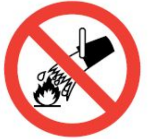
Do not extinguish with water
